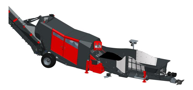
The Profit Pack compiles the two main characteristics of the LOGCUT MCS40: the possibility of resawing large volumes of wood on the one hand, and the versatility of a mobile machine on the other hand. This version was equipped with a grapple loading platform as well as an automated wood display system. The ergonomics of the workstation are studied in order to reduce the physical efforts of the operator to their minimum while maximizing the performance of the machine.
